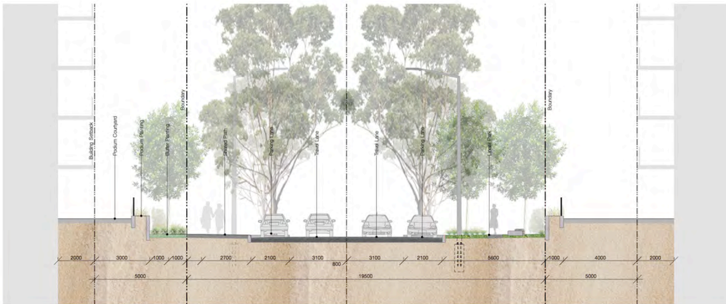
1A Type 2: Green Street Typical Section @1:100
